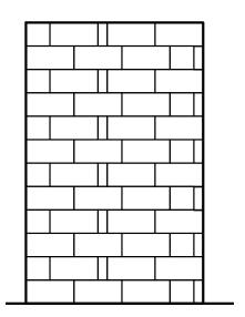
TO ACHIEVE 1, 2 AND 3 HOUR FIRE RATING: (PER ABOVE CHART PER CMU SIZE) APPLY 2 COATS OF AN EXTERIOR 100% STYRENE ACRYLIC PRIMER, THEN 50 MIL THICKNESS (DRY) OF ForceField® FireGuard® E-84 TO EXPOSED AND UNEXPOSED SIDE OF CMU WALL ASSEMBLY. ONCE COMPLETELY DRY, ASSEMBLY CAN BE TOP COATED WITH FLAT OR SEMI-GLOSS, WATER-BASED, LATEX PAINT.
