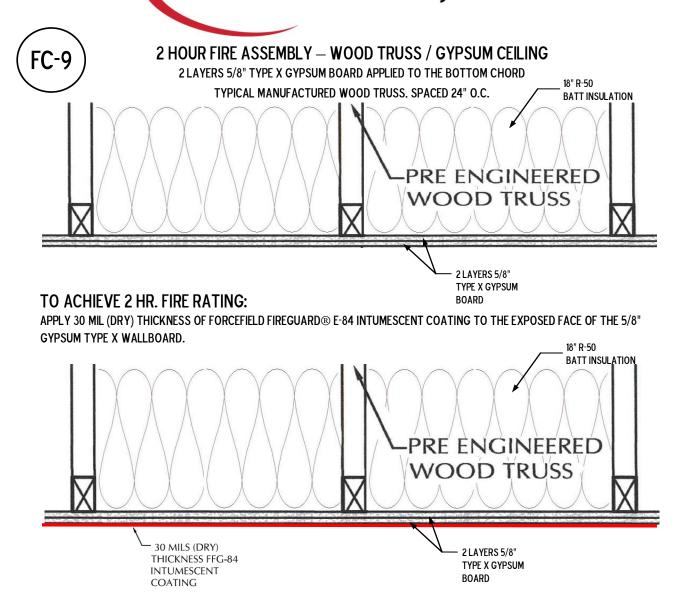
NOTE:  $2^{ND}$  Layer of 5/8" type x gypsum drywall needs to be attached with 2  $\frac{1}{2}$ " – 3" screws 8" o.c.
