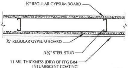
FIRE TEST ENDURANCE RATING: 2 HOUR STANDARD TESTED TO: ASTM E-119 FIRE TESTED LABORATORY: GUARDIAN FIRE TESTING LABORITORIES, INC. 480 HINMAN AVE. BUFFALO, NY 14216 REPORT NO: GL 71011 PRODUCT: ForceField® FireGuard® E-84 INTUMESCENT COATING (FFG E-84) MANUFACTURER: SHIELD INDUSTRIES, INC. 131 SMOKEHILL LANE WOODSTOCK, GA 30188
